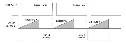
Figure 7-6 External Trigger Non-Overlap Exposure
