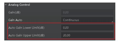
Figure 11-19 Set Gain under Once or Continuous Mode
