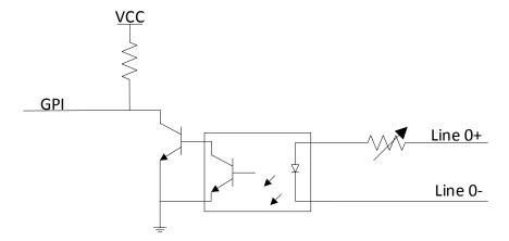
Figure 10-1 Line 0 Internal Circuit
