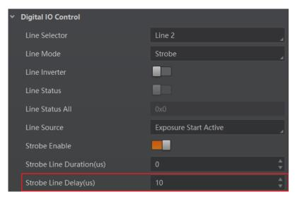
Figure 9-5 Set Strobe Line Delay
