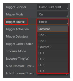
Figure 8-4 Set Trigger Source
