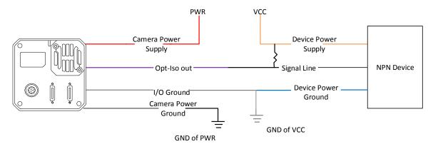
Figure 10-12 Line 1 Connecting to NPN Device
