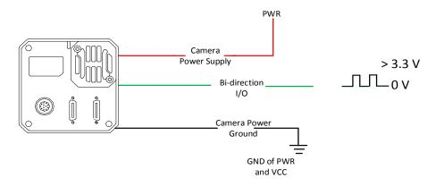
Figure 10-15 Line 2 Connecting to a Switch as Input
