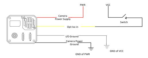
Figure 10-10 Line 0 Connecting to a Switch
