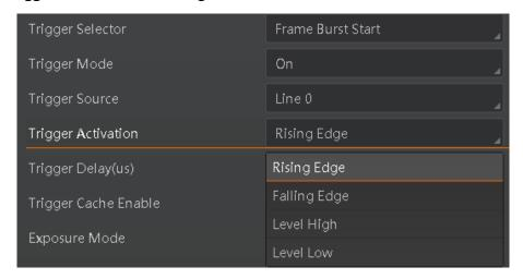
Figure 8-16 Set Trigger Activation
