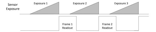
Figure 7-7 Internal Trigger Overlap Exposure
