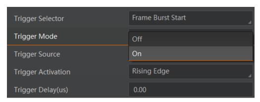
Figure 8-3 Set Trigger Mode
