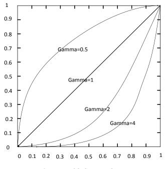
Figure 11-23 Gamma Curve
