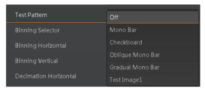
Figure 11-7 Set Test Pattern
