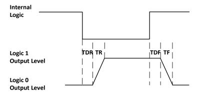
Figure 10-4 Output Logic Level
