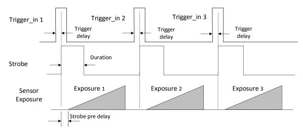
Figure 9-8 Sequence Diagram of Strobe Line Pre Delay
