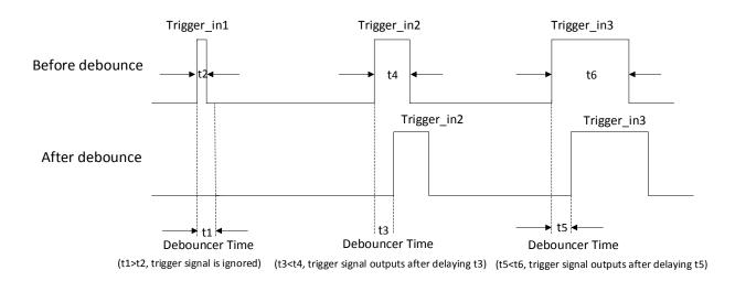
Figure 8-17 Trigger Debouncer Sequence Diagram
