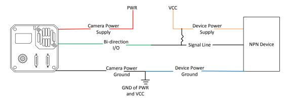
Figure 10-17 Line 2 Connecting to NPN Device as Output
