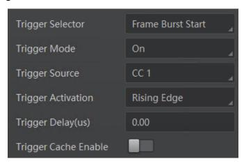
Figure 8-10 Set Frame Grabber Trigger
