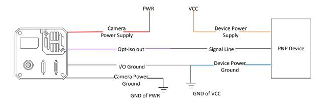
Figure 10-11 Line 1 Connecting to PNP Device
