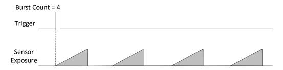
Figure 8-12 Sequence Diagram of Burst Frame Count
