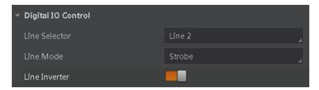
Figure 9-2 Enable Line Inverter
