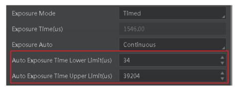
Figure 11-16 Set Exposure Time under Once or Continuous Mode
