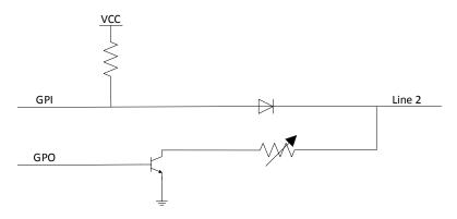
Figure 10-5 Line 2 Internal Circuit
