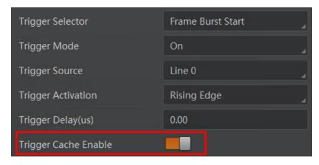
Figure 8-15 Enable Trigger Cache Enable
