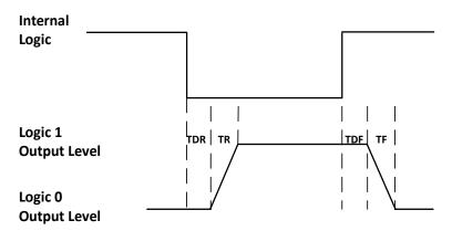
Figure 10-7 Output Logic Level
