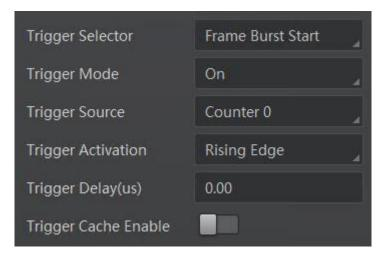
Figure 8-8 Set Counter Trigger
