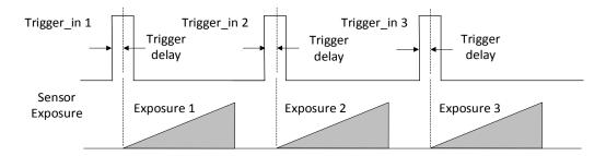
Figure 8-13 Signal Delay Sequence Diagram
