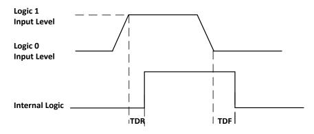
Figure 10-2 Input Logic Level
