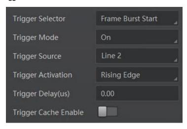
Figure 8-7 Set Hardware Trigger
