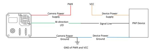
Figure 10-16 Line 2 Connecting to PNP Device as Output
