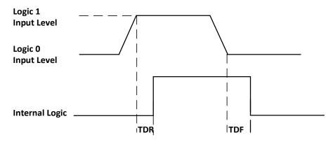
Figure 10-6 Input Logic Level
