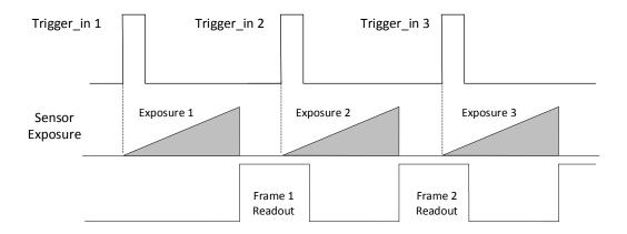
Figure 7-8 External Trigger Overlap Exposure
