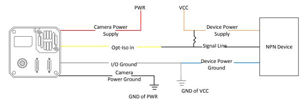
Figure 10-9 Line 0 Connecting to NPN Device
