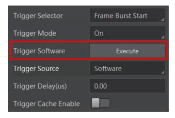
Figure 8-5 Set Software Trigger
