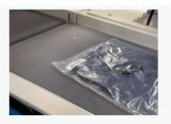
The code reader recognizes the parcel 2D code and does material sorting according to the barcode content. The solution solves the problem of distortion and folds in the code quality, efficient and stable recognition, and the reading rate reaches more than 99.9%.
