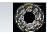
Lithium battery sealing welding defect detection: using deep learning algorithms for lithium battery sealing welding defect detection, can effectively detect welding defects such as welding offset, welding penetration, welding disconnection.
