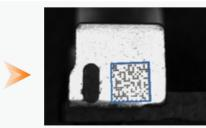
With the continuous upgrade of automated production line and engraving process, the size of QR code is getting smaller and smaller. ID series industrial readers with high resolution accessories ensure stable reading of very small codes.
