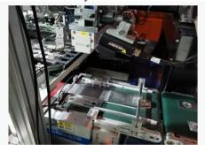
Battery top cover sheet DM code reading
