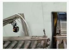
Automotive casting part code reading
