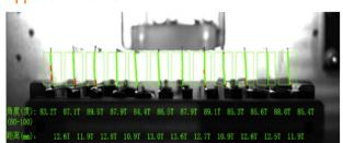
Li-ion battery lug measurement: Use the positioning and measurement module to measure the data related to Li-ion battery lugs, and design the software interface through secondary development.
