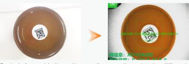
Bacteria ferment in the culture medium over time, showing different color changes in the test tube. the SC camera's ultra-high color reproduction can record the state changes of the culture medium in real time.
