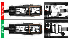
PV module junction box welding scar detection: using deep learning with traditional detection algorithms to detect PV module junction box welding scars.
