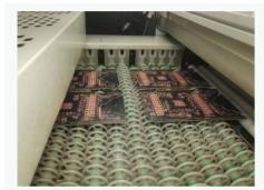
PCB board traceability code reading
