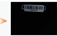
Intelligent logistics system is the connecting link between various systems, and the barcode information on the pallet is used to achieve battery tracking, management, status and other information. The solution's code is repeatedly used leading to easy dirty wear and low contrast, but the reading rate reaches more than 99.99%.
